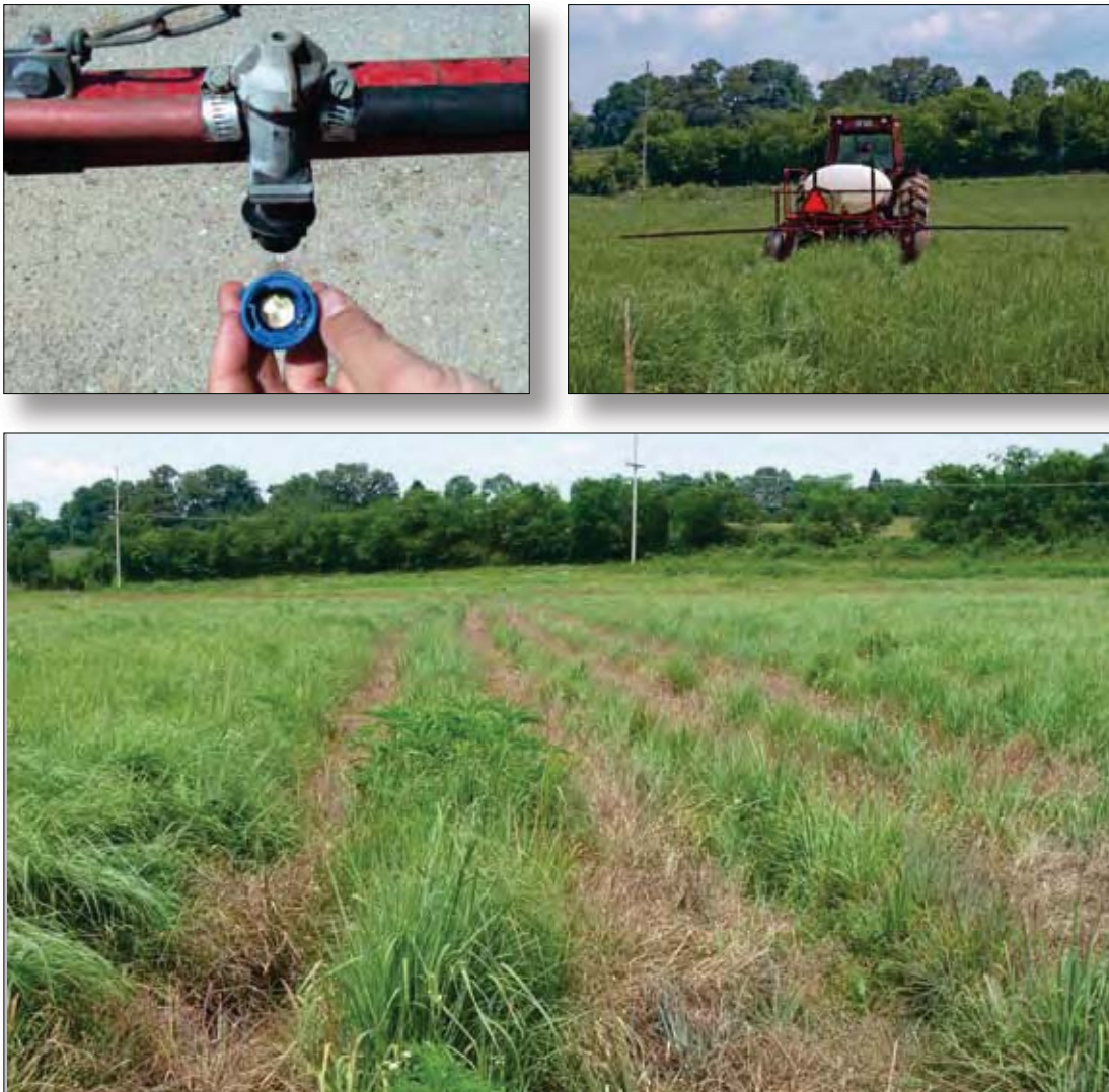
Fig 6.41–43 Strip-spraying can be accomplished by closing off every other or every third nozzle on the spray boom. This method can be used to effectively reduce grass density and intersperse forb cover.
