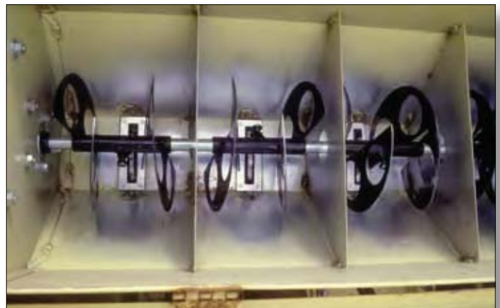
Fig. 5.23 and 5.24 Drills with “picker wheels” and agitators in the seed box (such as this Truax™) are recommended when planting bluestems and indiangrass. This ensures an even flow of seed and prevents seed lodging in the box.
